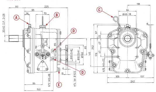
A Vent B Oil filler cap C Dipstick D Remote control bracket holes E Drain plug
